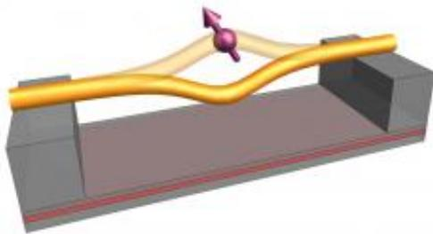
Schematic of a suspended carbon nanotube (CNT) containing a quantum dot filled with a single electron spin. The spin-orbit coupling in the CNT induces a strong coupling between the spin and the quantized mechanical motion  $u(z)$  of the CNT. Image (c) Prof. Dr. Guido Burkard, *Physics Review Letters* 108, 206811 (reproduced with permission)
