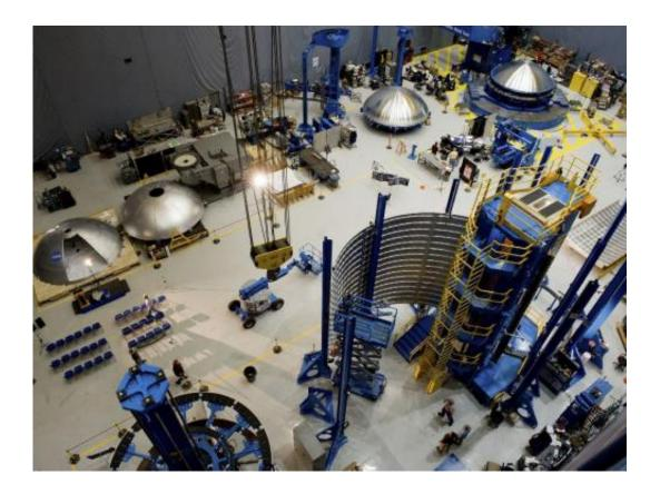
Four aluminum domes, created using innovative friction stir welding processes, are seen in this overhead view of the Marshall Space Flight Center Advanced Welding and Manufacturing Facility. Credit: NASA/MSFC/David Higginbotham
