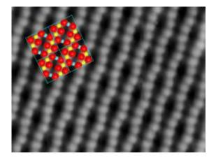
The oxygen atoms form wiggly lines on the surface, due to the atoms below (indicated in color)
