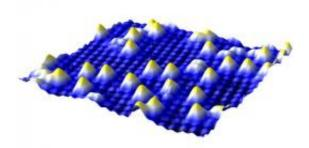
SMT-Image of the iron-oxide surface - with gold atoms on top
