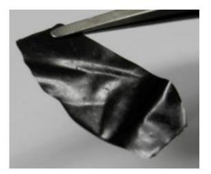
Yale engineers have developed a novel system for producing thin, conductive films. Pictured here, a freestanding carbon nanotube treated with one of the films.
