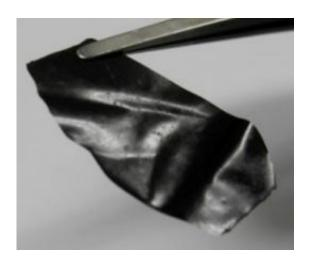
Yale engineers have developed a novel system for producing thin, conductive films. Pictured here, a freestanding carbon nanotube treated with one of the films.
