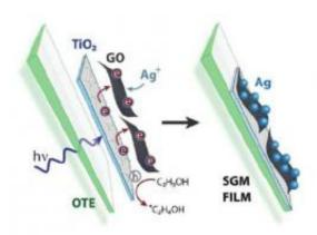
Under UV illumination, photogenerated electrons from the titanium dioxide are captured by the graphene oxide. The electrons "hop" to the other side of the graphene oxide and can reduce silver ions, resulting in the growth of silver nanoparticles. Image credit: Ian V. Lightcap, et al. ©2012 American Chemical Society
