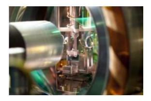
At the core of the experiment by Rainer Blatt's group in Innsbruck lies an optical resonator consisting of two highly reflective mirrors. Credit: Photo: C. Lackner
