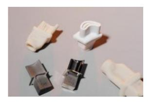
This image shows a collection of molds made through the large area maskless photopolymerization (LAMP) technology and airfoil components produced using them. Credit: Georgia Tech Photo: Gary Meek
