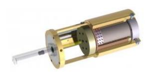
MIT-engineered device injects drug without needles, delivering a high-velocity jet of liquid that breaches the skin at the speed of sound. Image courtesy of the MIT BioInstrumentation Lab
