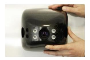
The 3-D camera in the flying robot can identify small objects measuring 20 by 15 centimeters from seven meters away. Credit: Fraunhofer IMS
