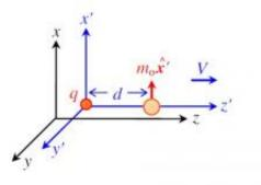
Charge-magnet paradox: the point electric charge q and the point magnetic dipole to its right are separated by distance d in the x'y'z' frame. An observer in the x'y'z' frame sees no torque, but a stationary observer in the xyz frame watching the x'y'z' system move with constant velocity along the z axis sees the moving electric charge exert a torque on the moving magnet. Image credit: Mansuripur. ©2012 American Physical Society
