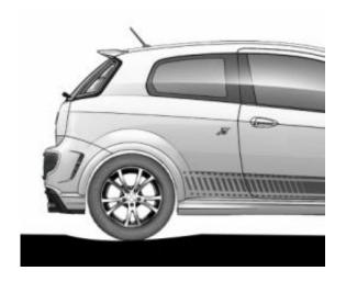
When the tires of a car or truck roll over a roadway, the maximum pavement deflection is just behind the path of travel. This has the effect of making the vehicle's tires roll continuously up a slight slope (exaggerated in this illustration), increasing the vehicle's fuel consumption. Image: Mehdi Akbarian
