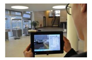
The virtual 3-D interior model of the building is displayed on the monitor. The location and the distance covered are marked in the map. Credit: Fraunhofer IPA
