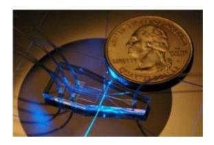
This is an assembled flow cytometry chip with size comparable to a US quarter. Credit: Tony Jun Huang, Penn State
