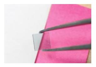
The image shows a sample of graphene oxide produced by the oxidation of epitaxial graphene on silicon carbide. Credit: Georgia Tech Photo: Gary Meek
