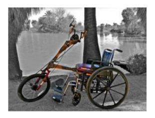
Both the hand-cycles and standard bicycles are made out of bamboo and recycled bike parts. Credit: BooGood Bicycles
