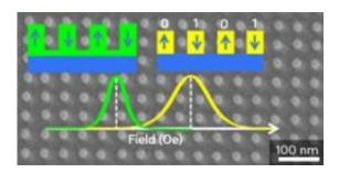
A magnetic film patterned into an array of dots (background) is known as a bitpatterned medium, and can store data at very high areal densities. Each dot requires a slightly different magnetic field to write or erase. Ranjbar and coworkers reduced this variation by adding a continuous layer underneath the dots, made of the same material as the dots themselves (green). By comparison, the traditional approach (yellow) had both a wider variation, and higher average switching fields. Credit: A\*STAR
