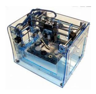
The Model 1 (above) is the first Fab@Home system. It includes everything necessary for basic, multimaterial desktop fabrication. It makes use of a basic "syringe pump"" material dispensing tool, with disposable syringes to enable dispensing of a wide variety of materials. Credit: Image courtesy of Fab@Home
