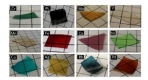
Samples of self-assembled metal-containing films made by the new sol-gel process. The films are essentially glass in which metal atoms are suspended, which imparts the color., Grid lines are 5 mm apart. Credit: Wiesner Lab
