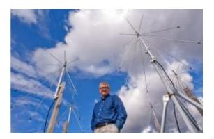
John Sahr with the passive radars on the roof of Sieg Hall. His group uses the radars to eavesdrop on FM radio stations in order to study the ionosphere. Credit: Mary Levin, UW Photography
