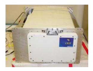
The picture above shows a mockup of a Polar unit. This mockup was used to verify the capability to achieve -80 degrees Celsius in Single Middeck Locker Equivalent format. Credit: NASA
