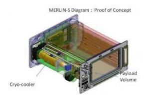
The image above shows a transparent diagram of a MERLIN. The Polars will be similar in design, but with increased volume capacity. Credit: NASA
