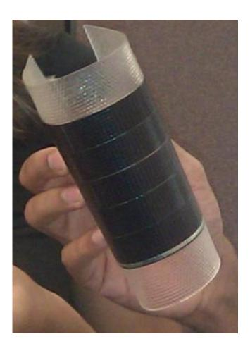
This is the high-efficiency Alta Devices solar cell. Credit: Joe Foster, Alta Devices
