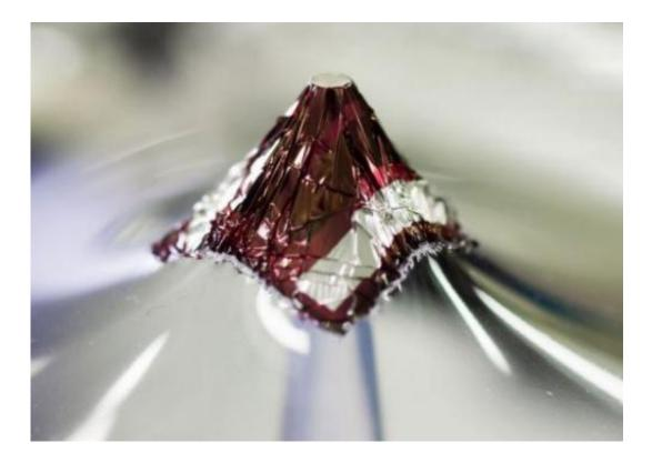
This undated recent picture, released by Nature Communications shows a thick ultrathin solar cell device attached to a elastomeric support, under threedimensional deformation by pressure from a plastic tube, developed by a team of Austrian and Japanese scientists. These solar cells are thinner than a thread of spider silk and flexible enough to wrap around a single human hair.
