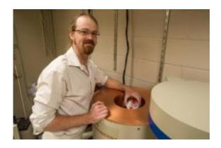
Dartmouth research associate Joshua Landis prepares to introduce a radioactive sample into a gamma-ray spectrometer. Credit: Eli Burak
