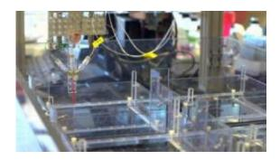
This computer-controlled system developed by biomedical engineering faculty members and students at Worcester Polytechnic Institute (WPI) is capable of continuous extrusion of microthreads with a range of diameters and quantities. Credit: Worcester Polytechnic Institute
