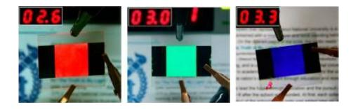
Red, green, and blue QLEDs, with the applied voltages in the upper left corner. The green QLED has a luminance of 168,000 candelas per square meter, which is more than three times higher than the previous best QLED brightness. Image credit: Jeonghun Kwak, et al. ©2012 American Chemical Society
