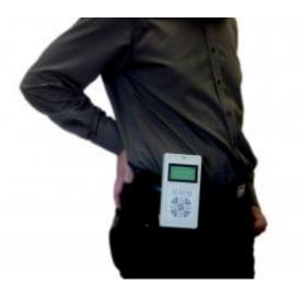
With the aid of magnetic coupling, power can be transmitted wirelessly from a transmitter to a receiver module. The prototype with the transmitter can be attached to the belt. Credit: Fraunhofer IKTS
