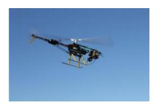
Remote-controlled robotic helicopter in flight with a laser-based greenhouse gas sensor extending from its nose. The aerial detector is easy to deploy, inexpensive to operate, can be guided by GPS, and provides measurements in both vertical and horizontal directions. Credit: Department of Civil and Environmental Engineering, Princeton University
