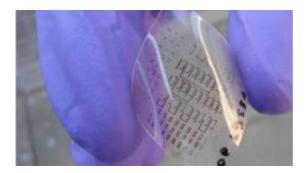
Printed electronic test circuit manufactured on a flexible plastic substrate at the Cavendish Laboratory, University of Cambridge. Credit: Enrico Gili
