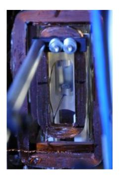
JILA's superradiant laser traps 1 million rubidium atoms in a space of about 2 centimeters between two mirrors. The atoms synchronize their internal oscillations to emit laser light. Credit: Burrus/NIST
