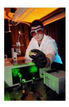
Georgia Tech graduate student Brandon Polander prepares for his FT-IR experiment. The green laser light is used to photo excite the spinach photosytem II sample. Credit: Georgia Tech Photo: Gary Meek
