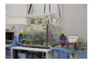
The first Galileo Full Operational Capability flight model payload with its solar panels in their 'boxed' position, being lifted by crane into its shipping container at Surrey Satellite Technology Ltd in Guildford, UK in April 2012. This is the first of 14 Galileo FOC payloads to be transported to prime contractor OHB in Germany for integration with their satellite platforms. Credits: SSTL 2012
