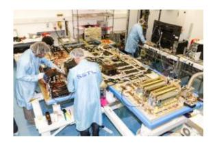
These payload panels for the first Galileo Full Operational Capability satellite are undergoing final testing in the Assembly Integration Test hall at Surrey Satellite Technology Ltd in Guildford, UK, in April 2012 before being boxed up for shipment to prime contractor OHB in Germany. Credits: SSTL 2012
