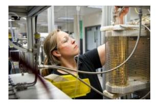
NREL Engineer Whitney Jablonski places a quartz reactor tube with a nickelbased catalyst into a reactor at NREL's Thermochemical Users Facility. Credit: Dennis Schroeder
