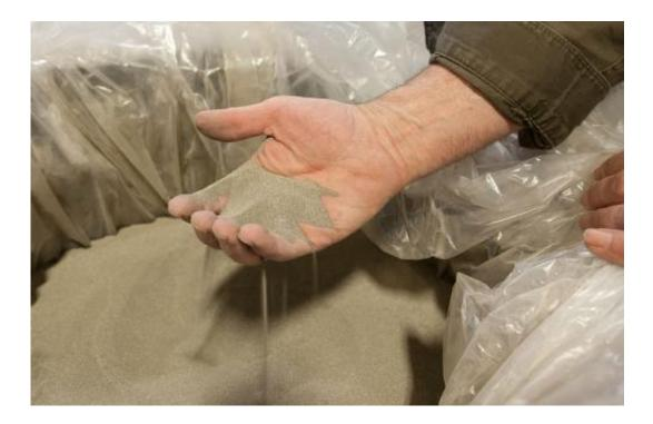
NREL makes its catalyst by mixing a nickel, magnesium, and potassium salt solution with a support structure created by CoorsTek. NREL's unique solution for a fluidizable tar reforming catalyst has been licensed by Rentech, Inc. Credit: Dennis SchroederCredit: Dennis Schroeder
