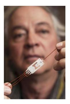
Sandia National Laboratories distinguished technical staff member Juan Elizondo-Decanini holds a prototype of a "neustristor," a new configuration for neutron generators that turns away from conventional cylindrical tubes in favor of the flat geometry of computer chips. He said the technology is ready to be licensed for some commercial applications, but more complex commercial applications could take five to 10 years. (Photo by Randy Montoya)
