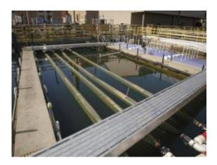
The NASA OMEGA floating photobioreactor prototype in a seawater tank at the Southeast wastewater treatment plant in San Francisco. The four flexible plastic tubes are filled with algae and wastewater, which circulates through the system. Credit: NASA Ames / Dominic Hart
