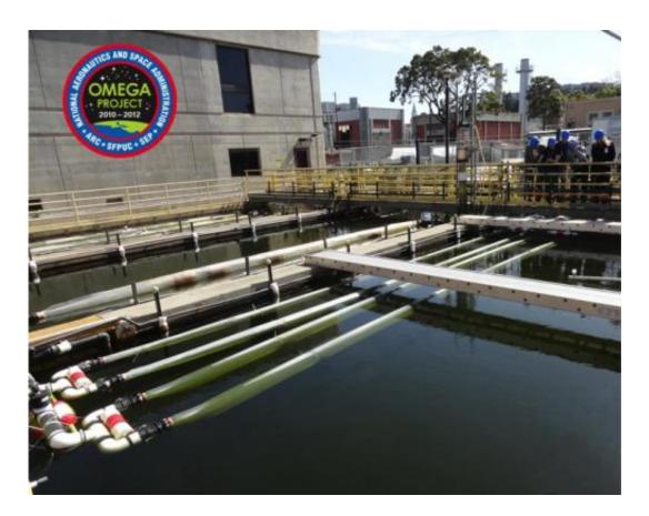
Wastewater with oil-producing algae circulate through photobioreactors (green tubes) floating in a seawater tank at the San Francisco Southeast Wastewater Treatment Plant, where NASA has set up one of its OMEGA research facilities.
