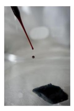
The superhydrophobic carbon nanotube sponge shows a remarkable ability to soak up oil from water. Researchers found that adding boron to the growth process creates covalent bonds in the nanotubes, making dense networks with robust qualities. (Credit: Jeff Fitlow/Rice University)
