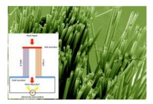
This image shows glass fibers coated with a thermoelectric material that generates electrical current when exposed to heat. The technology might be used to harvest energy from hot pipes or engine components, possibly representing a way to recover energy wasted in factories, power plants and cars. Credit: Purdue University photo/Scott W. Finefrock
