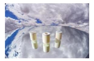
Sandia ear-plug-sized samplers, with silvery microvalves and solder connectors, seemingly hang poised to sample gases relevant to climate and weather. The prototype devices actually rest on a mirror, reflecting the day's Albuquerque weather. Credit: Photo by Randy Montoya, Sandia National Laboratories
