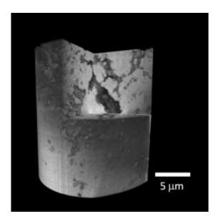
This 3D reconstruction of a lithium-ion battery electrode, composed of 1,441 individual images captured and aligned by the TXM, reveals nano-scale structural details to help guide future energy research.
