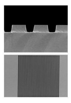
Top: The gratings are fabricated with approximately 700 nm between ridges. Each has slightly different spacing and thickness, affecting reflectivity and mechanical performance. Bottom: A single grating measuring 50 micrometers on a side.
