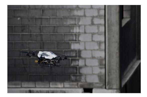
Within the framework of the EU project sFly, researchers at ETH Zurich have developed a new type of flying robot that can be navigated using only on-board cameras and a miniature computer. The micro helicopters require neither GPS nor remote control, thus reaching a new level of autonomy.
