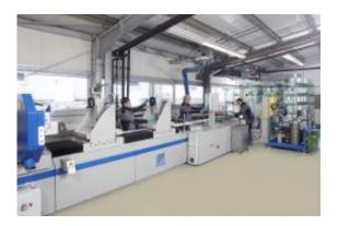
With the new system approach, CRP components can be produced "in assemblyline fashion." Credit: Fraunhofer ICT
