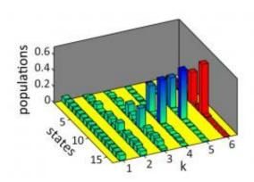
Quantum factorization of 143 using the adiabatic quantum algorithm. As the system evolves to its ground state k = 6, it reaches a superposition of states 6 and 9, which denotes the answers 11 and 13. Image credit: Xu, et al. ©2012 American Physical Society
