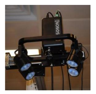
A hyperspectral line camera with four broadband light sources acquires images with the lens at center. A typical scan captures images at hundreds of discrete wavelengths that differ by as little as 2 nanometers.
