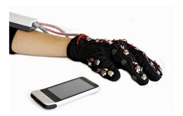
(Phys.org) -- People coping with the double absence of vision and hearing can communicate via mobile devices with the help of a special glove, now under development in Germany's Design Research Lab. The Mobile Lorm Glove is a wearable device that lets the user compose messages to be transmitted to the receiver's smartphone. This same glove allows the deaf-blind user to receive incoming messages as well. Basically, the person who cannot see or hear can use tactile feedback to
