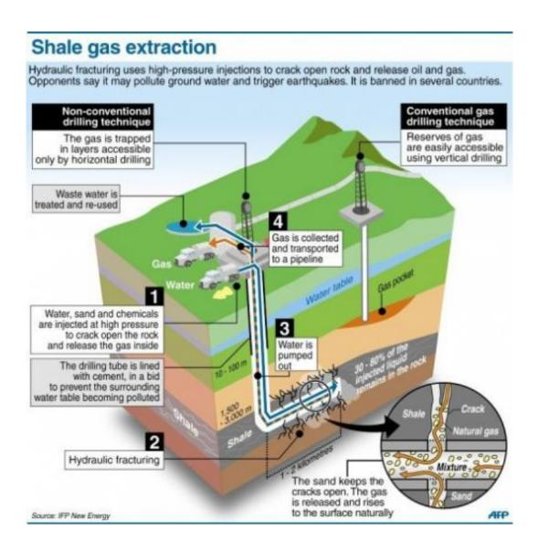
Explanation of the controversial technique of shale gas extractoin by hydraulic fracturing. Underneath the ground in southwestern Pennsylvania, bedrock is put under explosive pressure to fracture and spill out its lucrative cache of natural gas.
