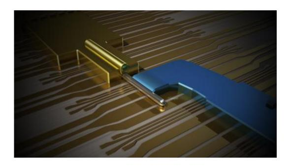
The device is made of an Indium Antemonide nanowire, covered with a Gold contact and partially covered with a Superconducting Niobium contact. The Majorana fermions are created at the end of the Nanowire. © TU Delft 2012
