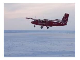
The ESA Twin-Otter leaving Alert in northern Canada on its way to rendezvous with NASA's P-3 aircraft over the Arctic Ocean. The Twin-Otter carries the ASIRAS radar altimeter, which is an airborne version of the instrument on the CryoSat satellite, and a laser scanner. Credits: ESA
