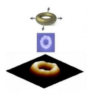
Illustration representing topography of a gold nanoring where a new method of sensing has been shown based on the damping of acoustic vibrations probed by transient absorption spectroscopy Copyright: A\*STAR
