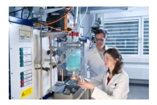
The first step towards the catalyst is the most important one: Julia Neuendorf and Malte Behrens control how a mixture of copper, zinc and aluminium salts precipitate the precursor for the catalyst of the methanol synthesis in the semi-automatic precipitation reactor. © Norbert Michalke for the MPG
